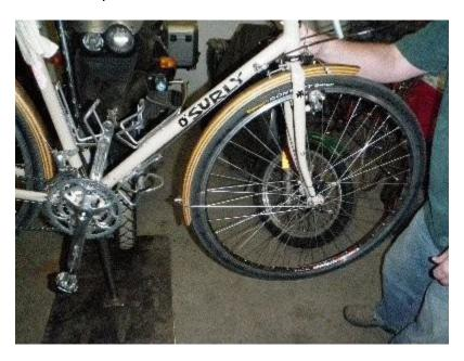
This is where we screw with you a little, if you read your instructions completely before you started you will have done this from the start. If you did not now it is time to completely remove the fenders you just spent an hour and a half to install and Silicon every hole and Loctite thread-locker every bolt.
