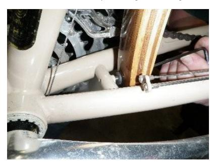
Mount 2 MK Fender standoffs to the frame eyelets at the rear dropouts. To do this you need to use 2 of the long set screws, 2 rubber washer, and 2 standoffs.
