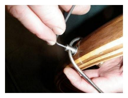
Line up your fender with the desired space between the tire and then mark your strut cuts. Remove the strut and cut and file the ends. Reinstall and make sure everything is aligned correctly. Personally, at this point, I would stop and drink a beer. The rear fender is mounted and it is time to look at the front.
