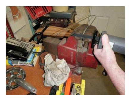
I would cut these about three inches from the end. That will be long, but it will give enough extra rod to work with. Mount the angle strut to the brake bridge. To do this you mount one custom MK Fender standoff to the brake bridge with a 5mm bolt and slide the angle strut through the hole and secure with a short set screw. This should look something like this:
