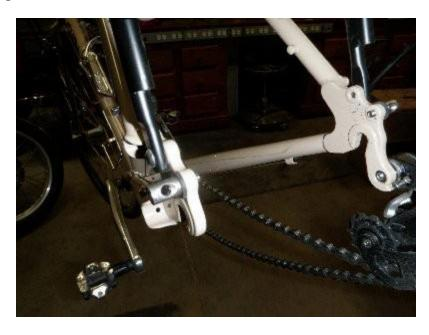
I would reinstall the rear wheel at this point. You need to install the rear fender strut and then estimate where to cut the strut ends.
