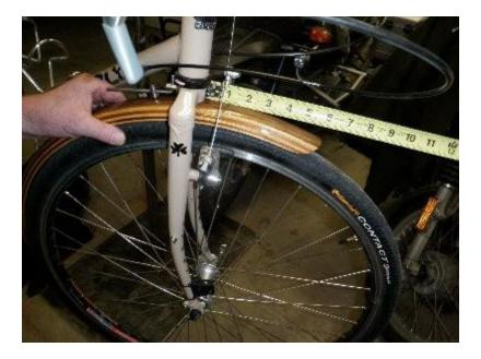
You have experience now that you have installed the rear fender so this should all be easy. Mount the angle strut to the fork crown and mount the 2 MK Fender standoffs to the fork eyelets. Decide where you want the fender strut to sit on the fender and mark your 2 holes. Drill and mount the MK Fender standoffs to the fender. Install the fender at the fork crown and install the fender strut. Mark your strut ends and cut them.
