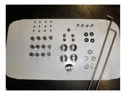
The first thing you need to do is cut the bent ends off your fender struts. Your strut will have one end that is extra long and have a 90 degree bend on it. These pieces are used to attach your fender to the frame at the brake bridge and fork crown.
